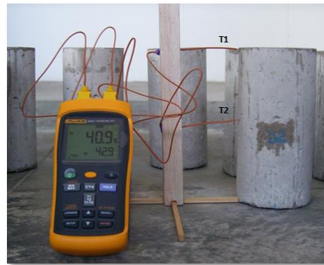
Figure 1. Accelerated attack on concrete samples: showing the temperature data acquisition.
